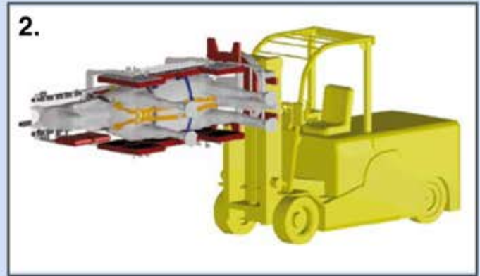
Surgery in combination with forklift: rotatable to lateral position left, right and dorsal, lifting in each working level
